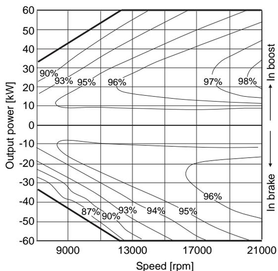
Fig. 10 Motor efficiency
