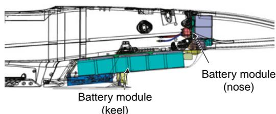
Fig. 3 Front collision test for FIA regulations and battery layout for RA109K
