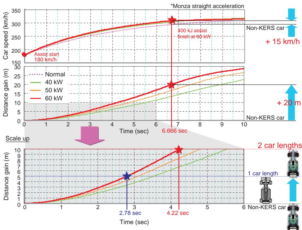
Fig. 2 Assist time / car speed and distance gain
