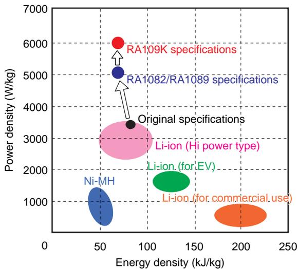
Fig. 13 Battery specifications
