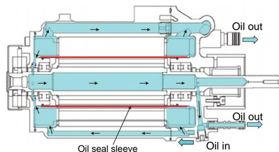
Fig. 9 Section of motor with cooling oil flow
