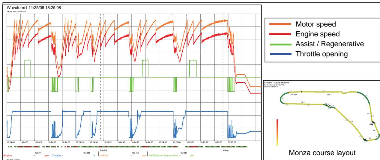
Fig. 19 Circuit mode test on dyno
