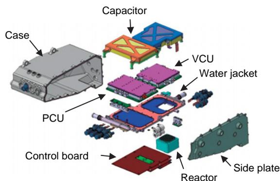
Fig. 12 View of PCU for race specification
