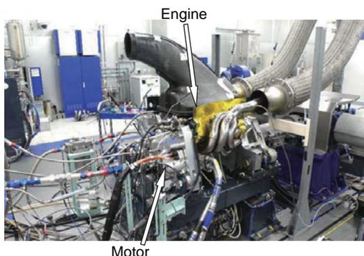
Fig. 18 Combination examination of engine and motor
