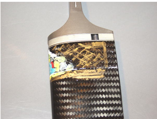
Figure 9. “disbond” revealed by UT examination
